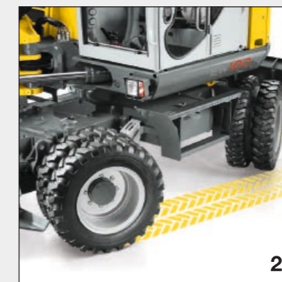
All-wheel steering for a particularly small turning circle.
